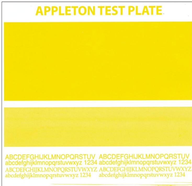
Pre-print testing is performed using similar line anilox and identical graphical formatting helping to keep results consistent between evaluations.
